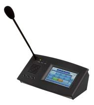
**PPM-IT5:** The 3 hardware keys can be freely assigned by software. The PPM-IT5 Media console is a versatile device that enhances paging over IP-networking.
