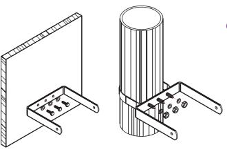
**1.** Remove the "U" bracket from the speaker. Align the bracket and mark the fixing points. Fix the bracket using suitable fixings (Not supplied).
