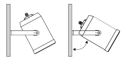
**6.** Re-fit the speaker to the "U" bracket. Position the speaker to the desired angle then tighten the fixings to secure in place.
