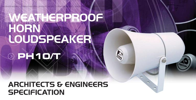
The unit shall be the PENTON model PH10/T or equal and approved. The horn enclosure shall be constructed of high impact ABS with UV inhibitors and non-perishable gaskets to prevent the ingress of water or dust and be rated to a minimum of IP66. The unit will be mounted via a stainless steel "U" bracket and fixings. The speaker assembly shall comprise of a high-density phenolic resin diaphragm housed in a flared chamber, 200mm long x 138mm diameter.
