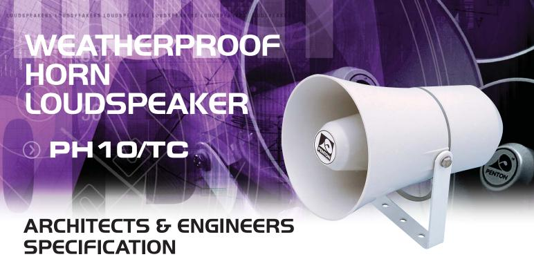
The unit shall be the PENTON model PH10/TC or equal and approved. The horn enclosure shall be constructed of high impact ABS with UV inhibitors and non-perishable gaskets to prevent the ingress of water or dust and be rated to a minimum of IP66. The unit will be mounted via a stainless steel "U" bracket and fixings. The speaker assembly shall comprise of a high-density phenolic resin diaphragm housed in a flared chamber, 200mm long x 138mm diameter.
