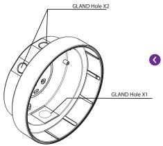
**1.** Decide on the back box orientation. Normally the back box is installed with the 2 x 20mm knockouts facing upwards. However the back box can be installed in any orientation as well as horizontally on a ceiling if required.
