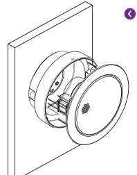
**4.** Once the back box has been fixed securely to the surface the installation cable can be fitted as required. The cable can then be terminated into the terminal block fitted to the back box. The terminals are suitable to take "loop in" "loop out" connections up to 2.5mm per core.
