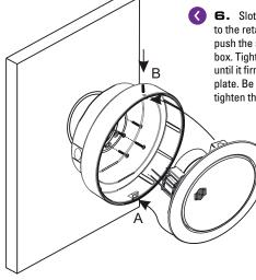
**G.** Slot the speaker plate on to the retaining lug 'A' and then push the speaker into the back box. Tighten the grub screw 'B' until it firmly holds the speaker plate. Be careful not to over tighten the grub screw.
