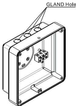
1. Decide on the back box orientation. Normally the back box is installed with the 3 x 20mm knockouts facing upwards. However the back box can be installed in any orientation as well as horizontally on a ceiling if required.
