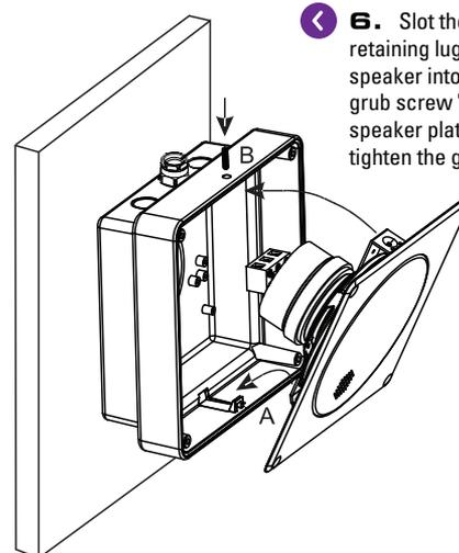
6. Slot the speaker plate on to the retaining lug "A" and then push the speaker into the back box. Tighten the grub screw "B" until it firmly hold the speaker plate. Be careful not to over tighten the grub screw.
