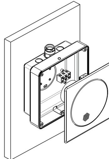
4. Once the back box has been fixed securely to the surface the installation cable can be fitted as required. The cable can then be terminated into the terminal block fitted to the back box. The terminals are suitable to take "loop in" "loop out" connections up to 2.5mm per core.
