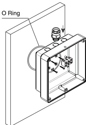
2. The back box has the option of glanding cable directly into any of the 3 x 20mm knockouts or through the rear of the cabinet.
